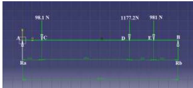
Fig. 2 steering assembly weight, driver's cabin weight and transmission assembly weight distribution diagram
